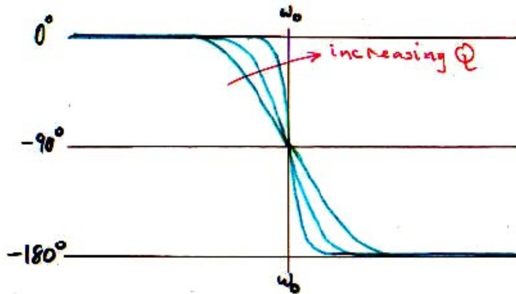
Increased  $Q$  causes sharper phase change between the  $0^\circ$  and  $-180^\circ$  asymptotes.
