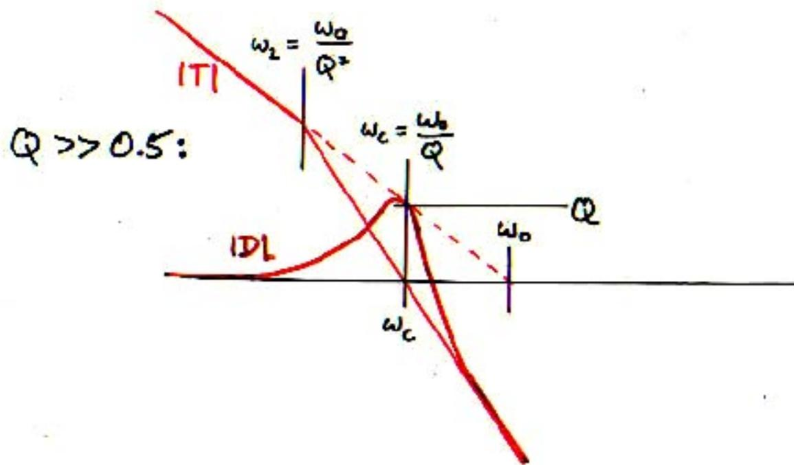
Hence: discrepancy factor  $D$  peaks if second pole is not sufficiently far above  $\omega_0$ , and  $D$  is characterized by the  $Q$ -factor of its quadratic, which is related to  $\omega_2$  (and  $\omega_0$ ) by  $Q = \sqrt{\frac{\omega_0}{\omega_2}}$ .
