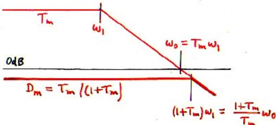
$$T = T_m \frac{1}{1 + \frac{s}{\omega_1}} = \frac{1}{\frac{s}{\omega_0} \left( 1 + \frac{\omega_0}{T_m s} \right)}$$
