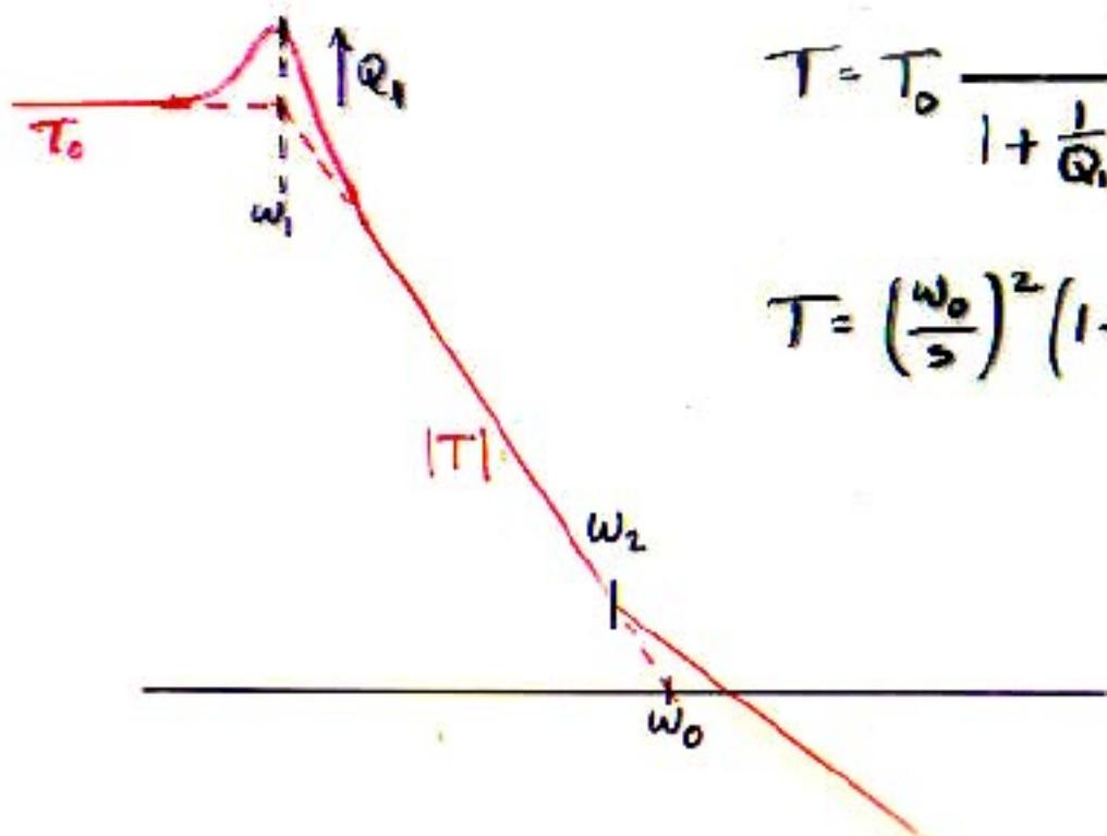
$$T = T_0 \frac{1 + \frac{s}{\omega_2}}{1 + \frac{1}{Q_1} \left( \frac{s}{\omega_1} \right) + \left( \frac{s}{\omega_1} \right)^2}$$
