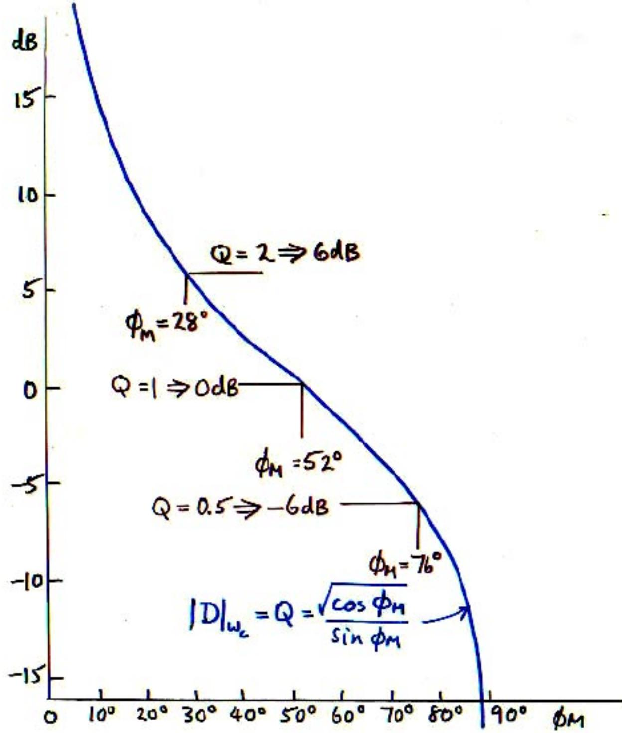
A phase margin  $\phi_m$  less than  $76^\circ$  causes complex roots in  $D$ , and therefore in the closed-loop gain  $G$ . In the frequency domain, this results in peaked high-frequency response; in the time domain, it results in transient overshoot. For constant  $G_\infty$ ,  $G \propto D$  and the response to a step input is
