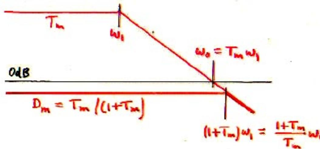
$$T = T_m \frac{1}{1 + \frac{s}{\omega_1}} = \frac{1}{\frac{s}{\omega_b} \left(1 + \frac{\omega_0}{T_m s}\right)} \xrightarrow{T_m \rightarrow \infty} \frac{1}{\frac{s}{\omega_b}}$$
