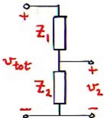
$$\frac{v_2}{v_{\text{tot}}} = \frac{Z_2}{Z_1 + Z_2}$$
