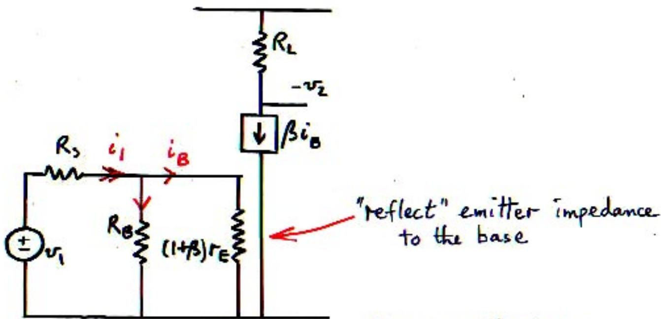
$$i_1 = \frac{v_1}{R_s + R_B \parallel (1+\beta)r_E}$$
