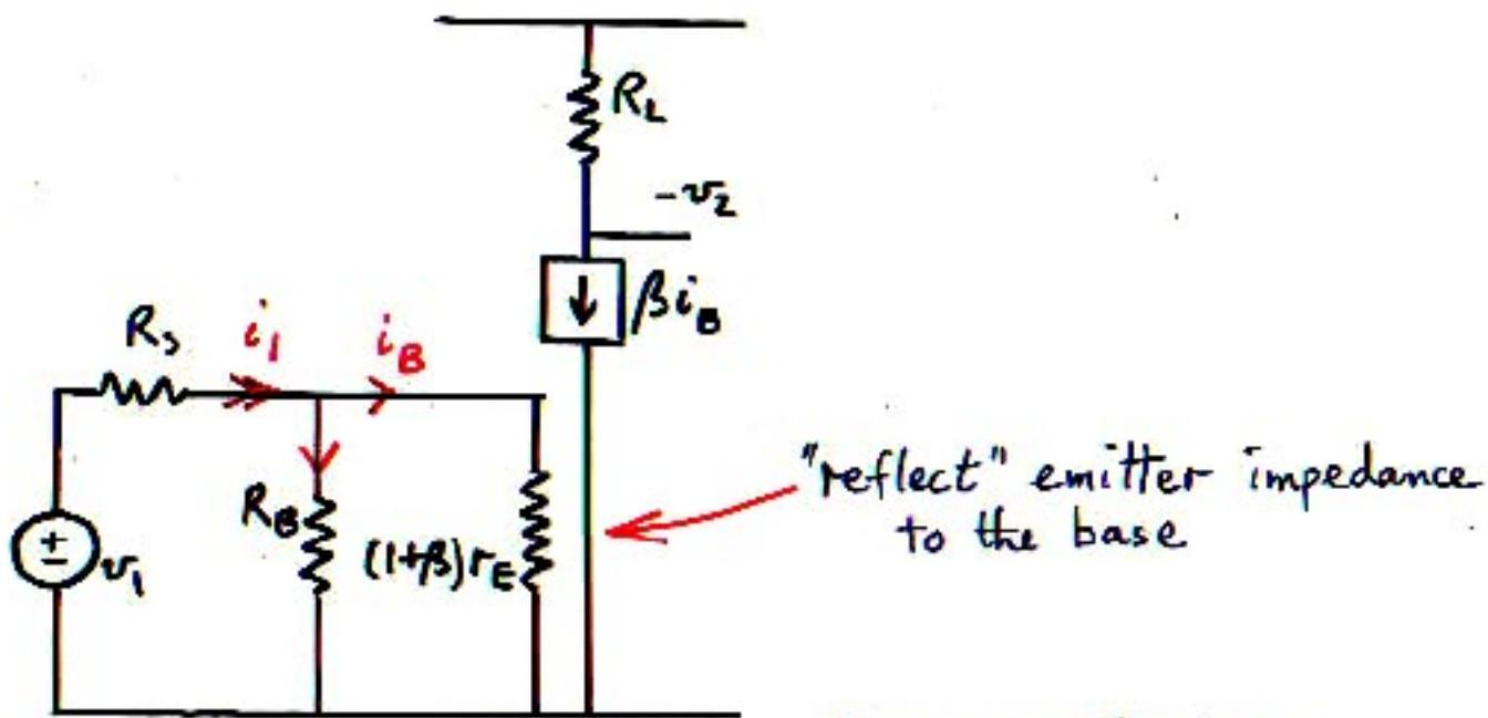
$$i_1 = \frac{v_1}{R_s + R_B \parallel (1+\beta)r_E}$$
