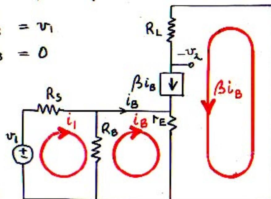
Finally,  $v_2 = R_L \beta i_B$
