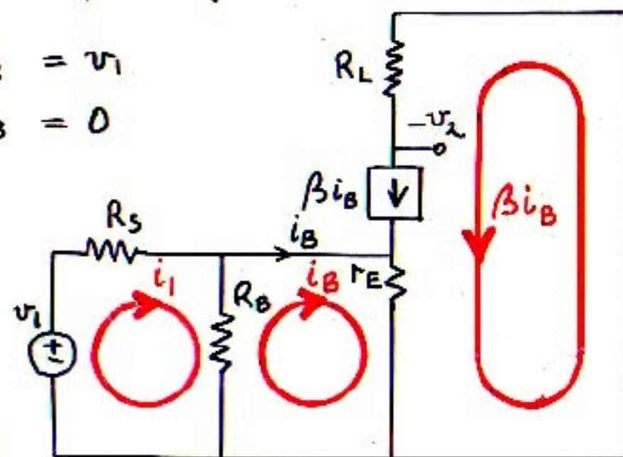
Finally,  $v_2 = R_L \beta i_B$
