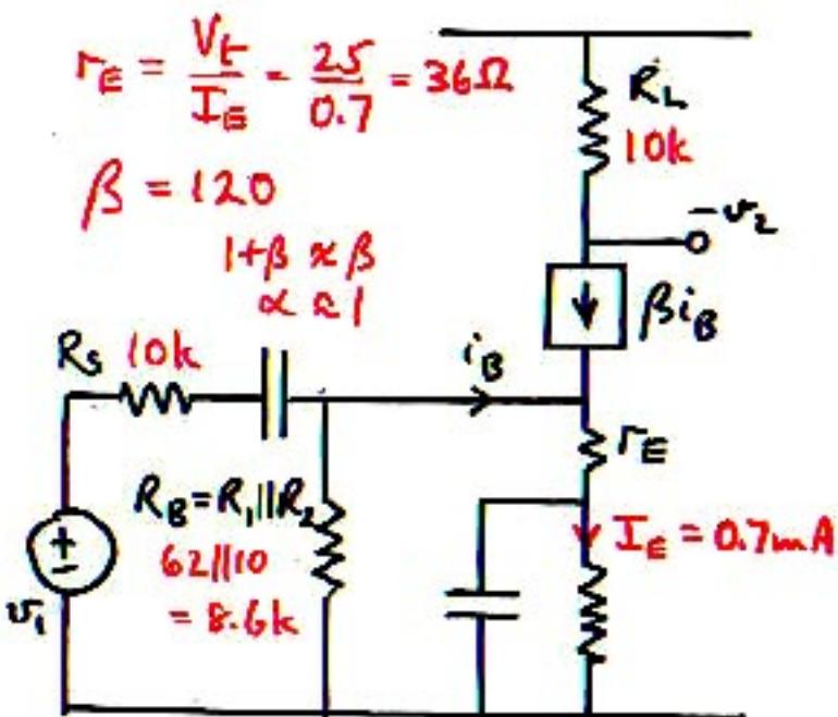
$$A_m = \frac{R_B}{R_s + R_B} \cdot \frac{\alpha R_L}{r_E + (R_s \parallel R_B)(1 + \beta)}$$
