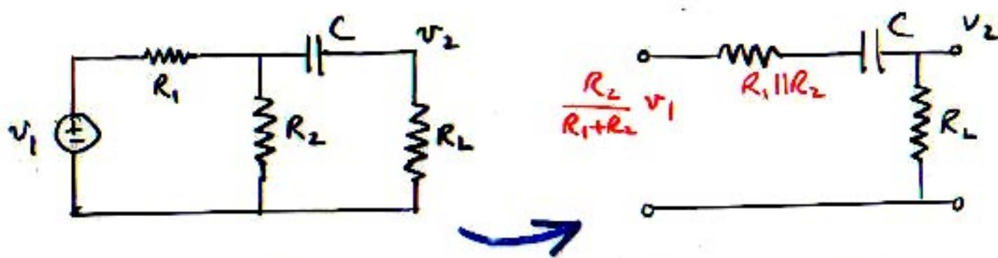
This is how element groupings arise naturally, by circuit reduction through successive loop and node removal.
