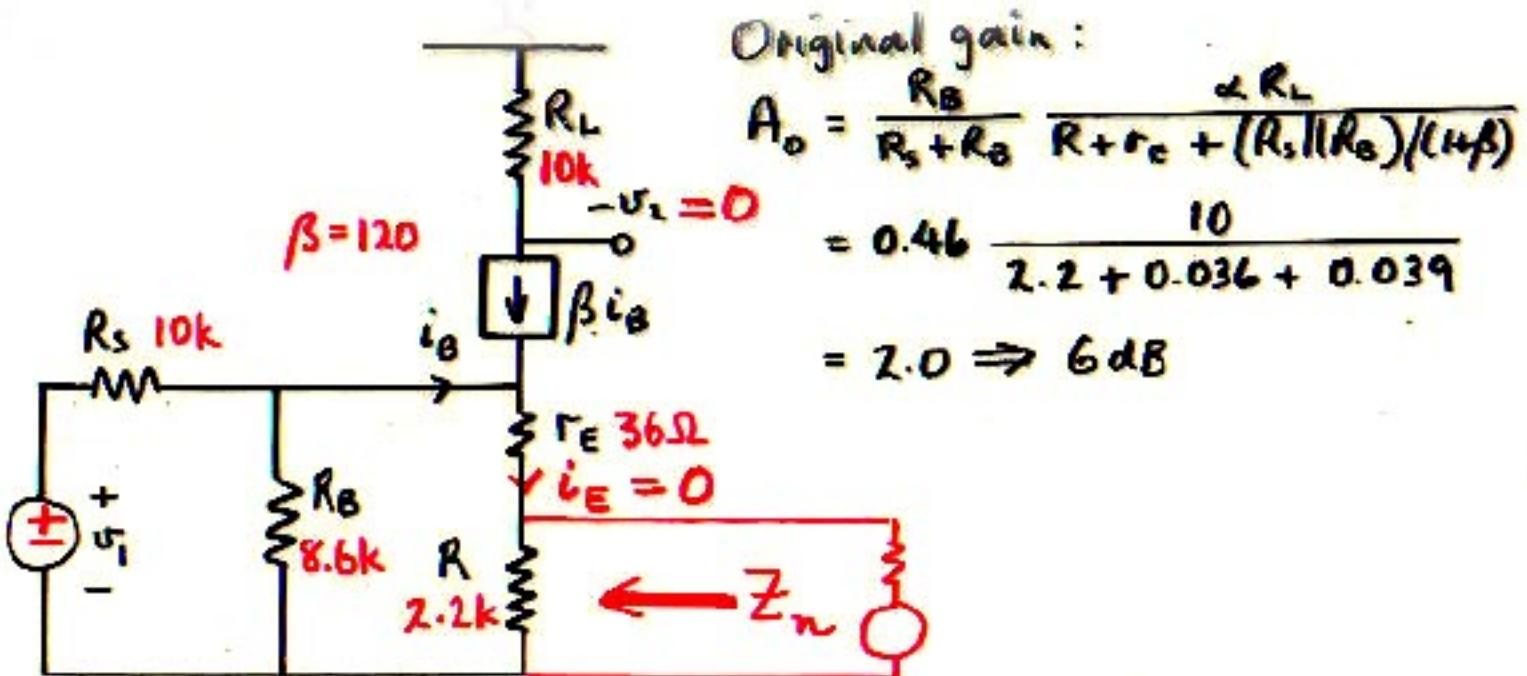
Step 2. Calculate  $Z_n$  by applying a second injected signal across  $R$ , and adjusting it with respect to  $v_i$  to null  $v_{o1} = v_2 = 0$ . Then, since  $v_2 = 0$ ,  $i_E = 0$ , hence:
