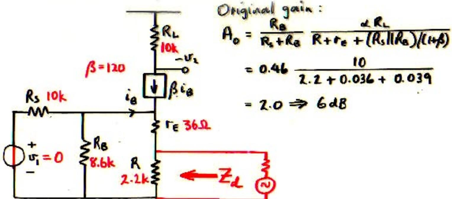
Step 1. Calculate  $Z_d$  by shorting  $u_{c1} = u_i$ , and applying a second injected signal across  $R$ :
