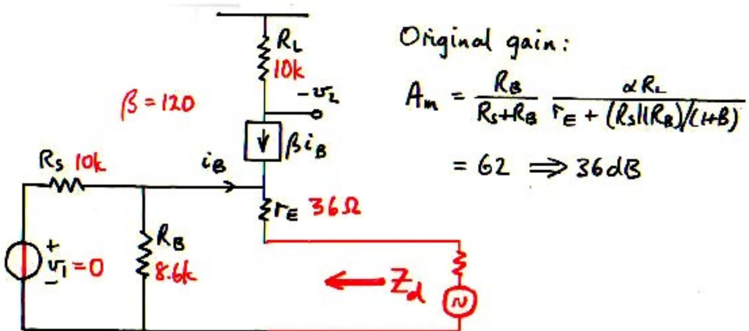
Step 1. Calculate  $Z_d$  by shorting  $v_{i1} = v_i$  and applying a second injected signal in series with  $r_E$ :
