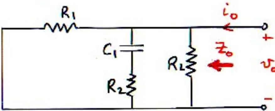
Find the output impedance  $Z_o = v_o / i_o$  by designating  $C_1$  as an "extra" element.
