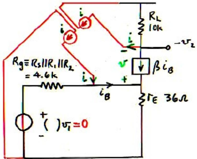
A separate ground can be identified for each current generator  $i$ .
