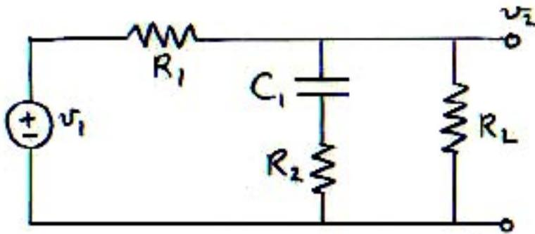
Find the transfer function  $A = v_2/v_1$  by designating  $C_1$  as an "extra" element.
