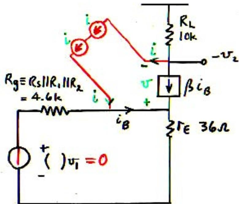
The current generator  $i$  can be divided into two equal current generators in series.
