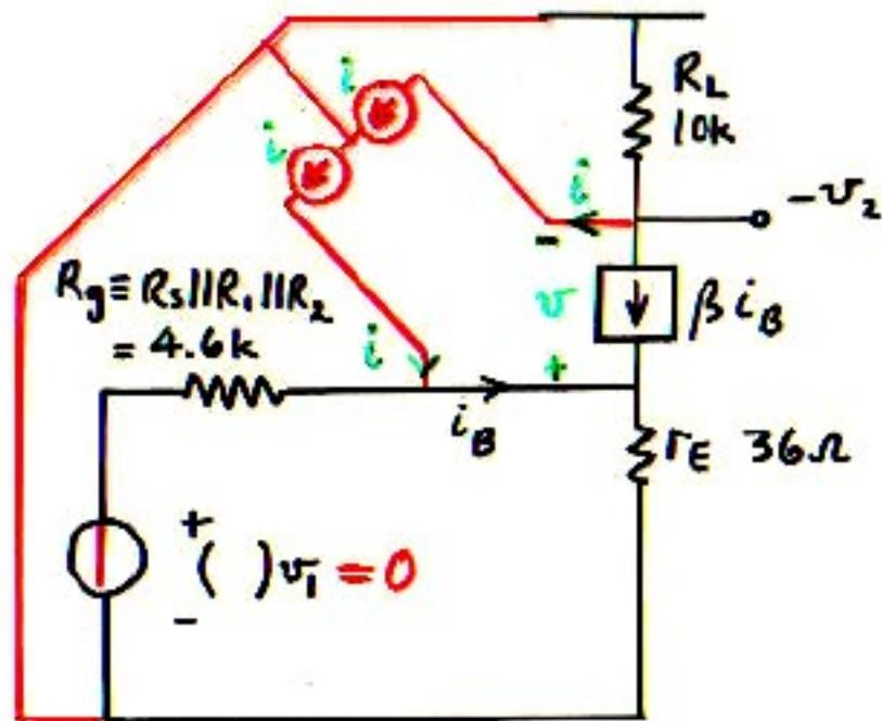
The current generator  $i$  can be divided into two equal current generators in series.
