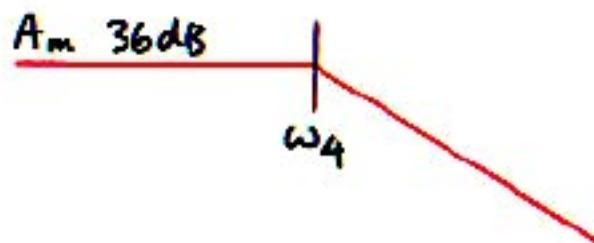
Since the midband gain  $A_m = 36\text{dB}$  has already been determined, use the Extra Element Theorem to find the correction factor resulting from inclusion of  $Z \rightarrow 1/sC_t$ .
