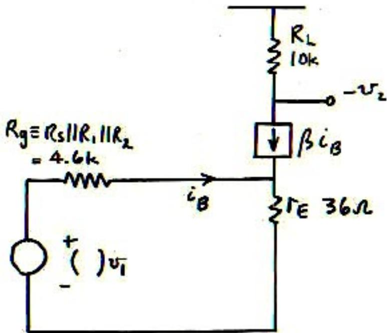
Midband model after Thevenin reduction of  $R_s, R_1, R_2$ :
