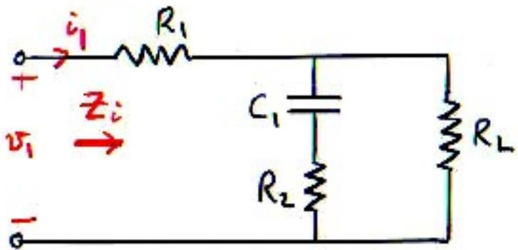
Find the input impedance  $Z_i = v_i / i_1$  by designating  $C_1$  as an "extra" element.
