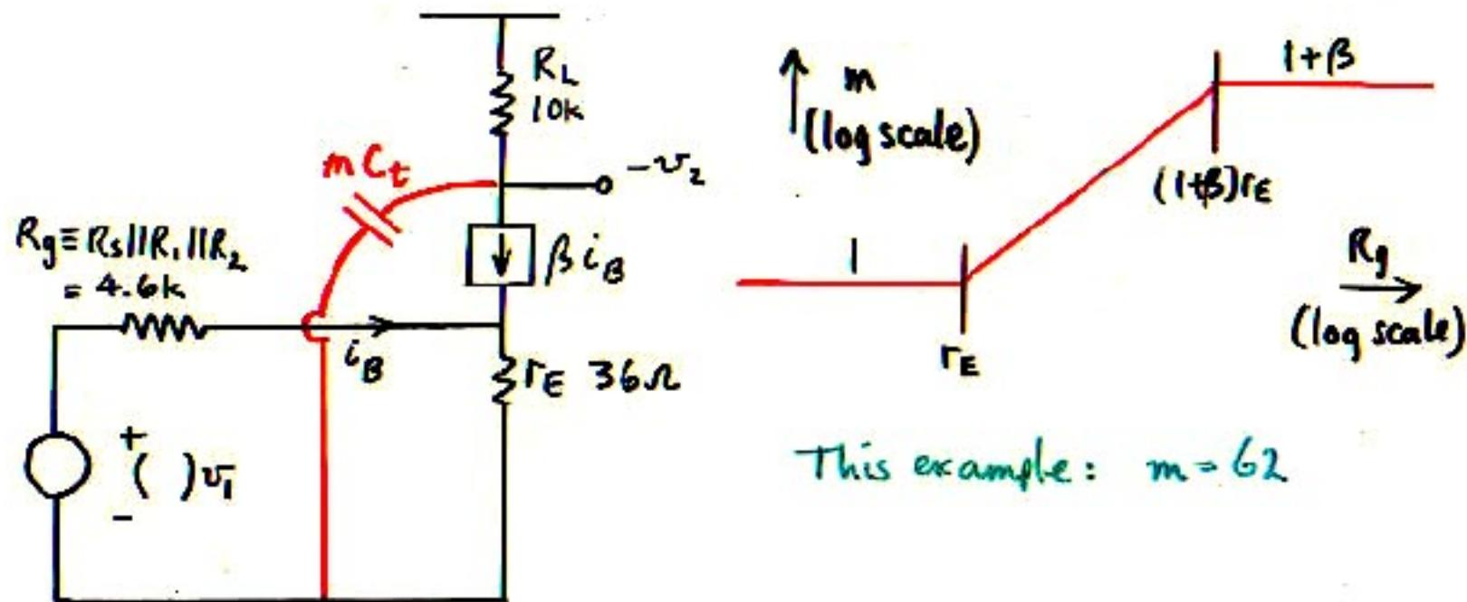
Midband model after Thevenin reduction of  $R_s, R_1, R_2$ :
