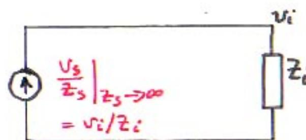
$$z_i = \frac{v_s | z_s \rightarrow 0}{v_s | z_s \rightarrow \infty} = \frac{v_s | z_s \rightarrow 0}{v_L z_s | z_s \rightarrow \infty} = \frac{1/A | z_s \rightarrow 0}{z_s A | z_s \rightarrow \infty} = \frac{z_s A | z_s \rightarrow \infty}{A | z_s \rightarrow 0}$$
