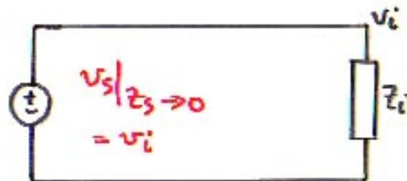
$$\frac{v_i}{v_i/z_i} = z_i = \frac{v_s | z_s \rightarrow 0}{v_s | z_s \rightarrow \infty}$$
