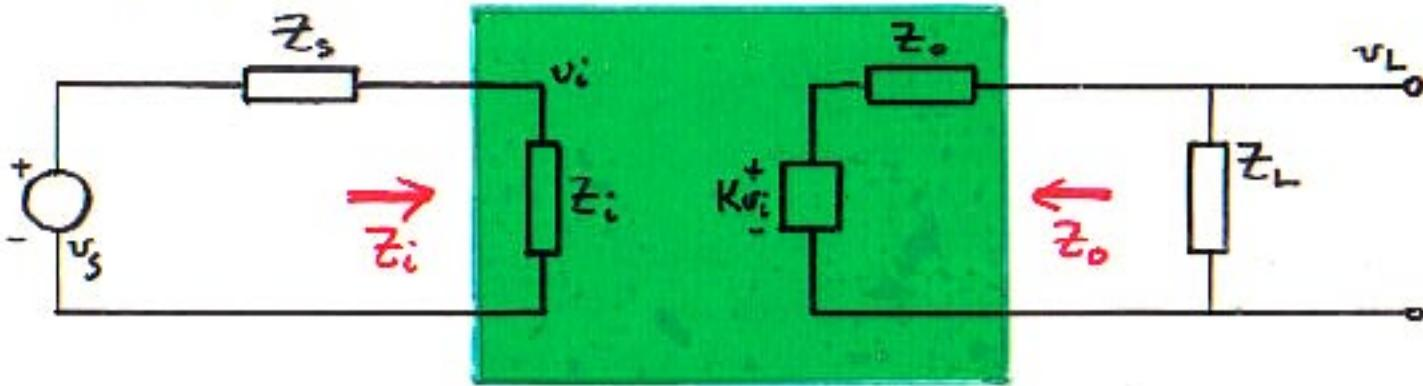
Result for "inside" input and output impedances:
