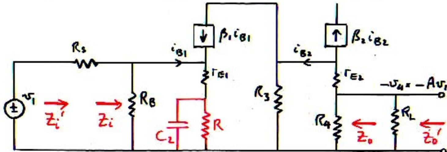
$$A_m = \frac{R_B}{R_B + (1+\beta_1)r_{E1}} \cdot \frac{\beta_1 R_B}{R_s + R_B \parallel (1+\beta_1)r_{E1}} \cdot \frac{R_4 \parallel R_L}{R_4 \parallel R_L + r_{E2} + R_3/(1+\beta_2)}$$
