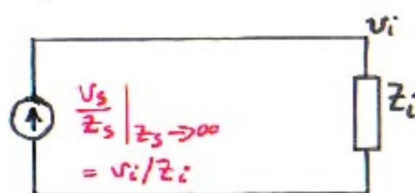
$$\frac{v_i}{v_i/z_i} = z_i = \frac{v_s | z_s \rightarrow 0}{\frac{v_s}{z_s} | z_s \rightarrow 00}$$
