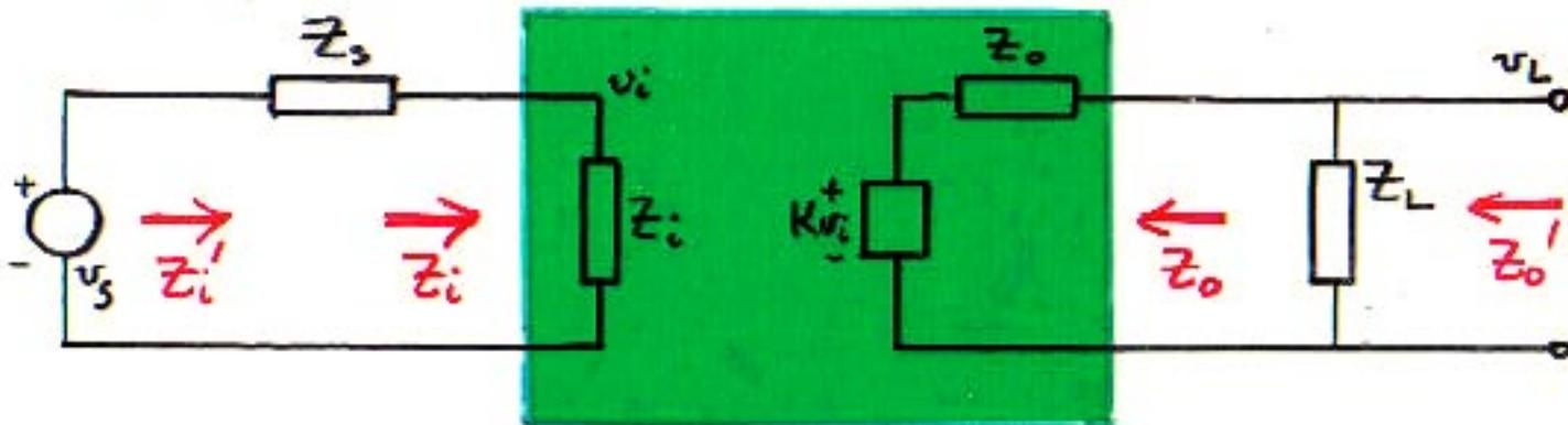
Result for "inside" input and output impedances:
