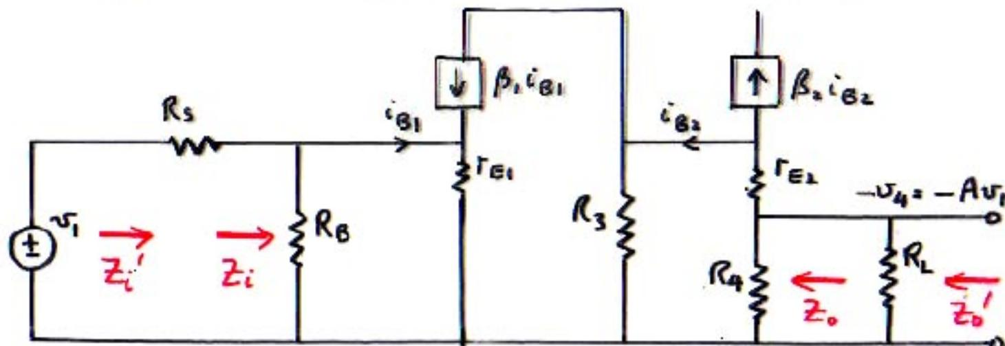
$$A_m = \frac{R_B}{R_B + (1+\beta_1)r_{E1}} \cdot \frac{\beta_1 R_B}{R_s + R_B \parallel (1+\beta_1)r_{E1}} \cdot \frac{R_4 \parallel R_L}{R_4 \parallel R_L + r_{E2} + R_3/(1+\beta_2)}$$
