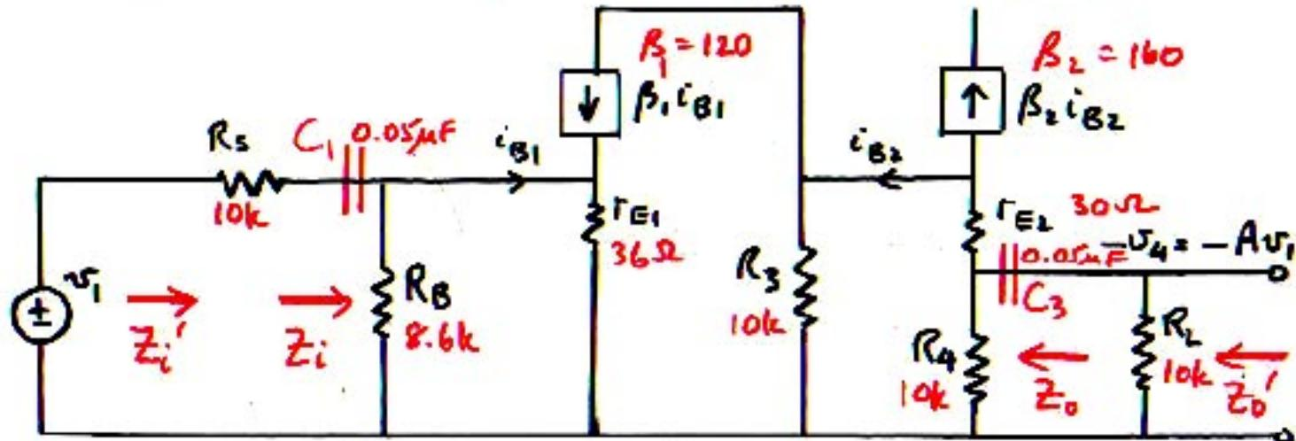
$$A_m = \frac{R_B}{R_B + (1+\beta_1)r_{E1}} \cdot \frac{\beta_1 R_B}{R_s + R_B || (1+\beta_1)r_{E1}} \cdot \frac{R_4 || R_L}{R_4 || R_L + r_{E2} + R_3 / (1+\beta_2)}$$
