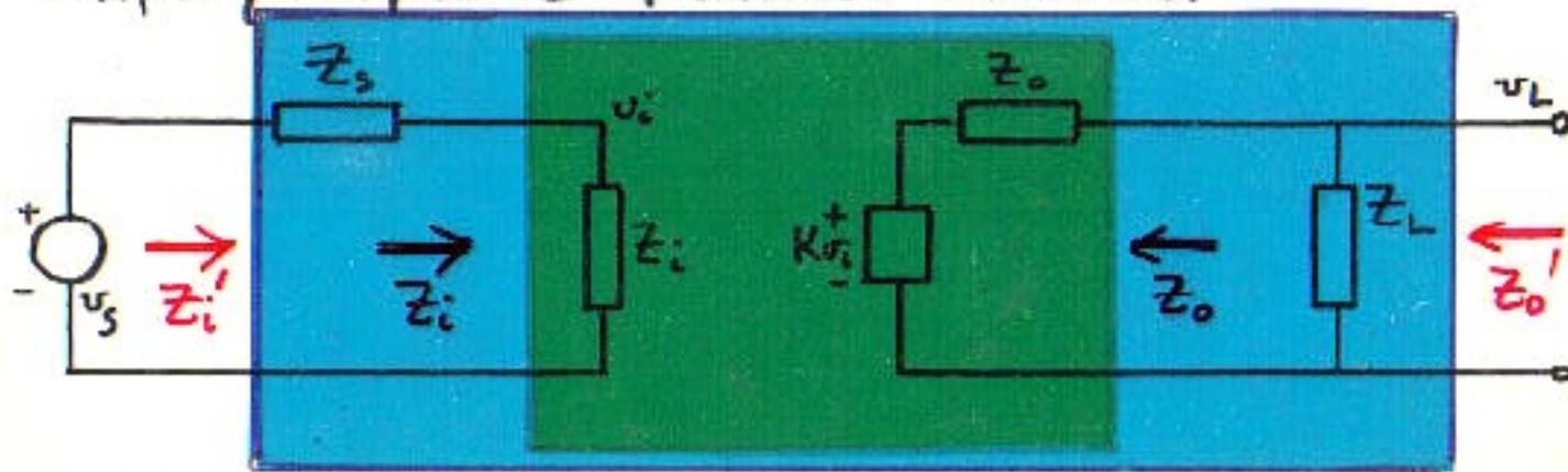
Result for "inside" input and output impedances:
