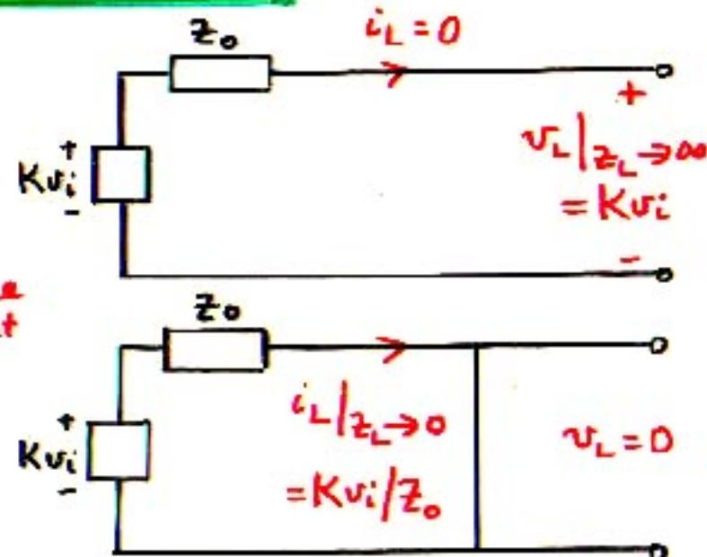
$$z_0 = \frac{v_L|_{z_L \rightarrow \infty}}{i_L|_{z_L \rightarrow 0}} = \frac{\frac{v_L}{v_s}|_{z_L \rightarrow \infty}}{\frac{v_L}{v_s z_L}|_{z_L \rightarrow 0}} = \frac{A|_{z_L \rightarrow \infty}}{\frac{A}{z_L}|_{z_L \rightarrow 0}}$$
