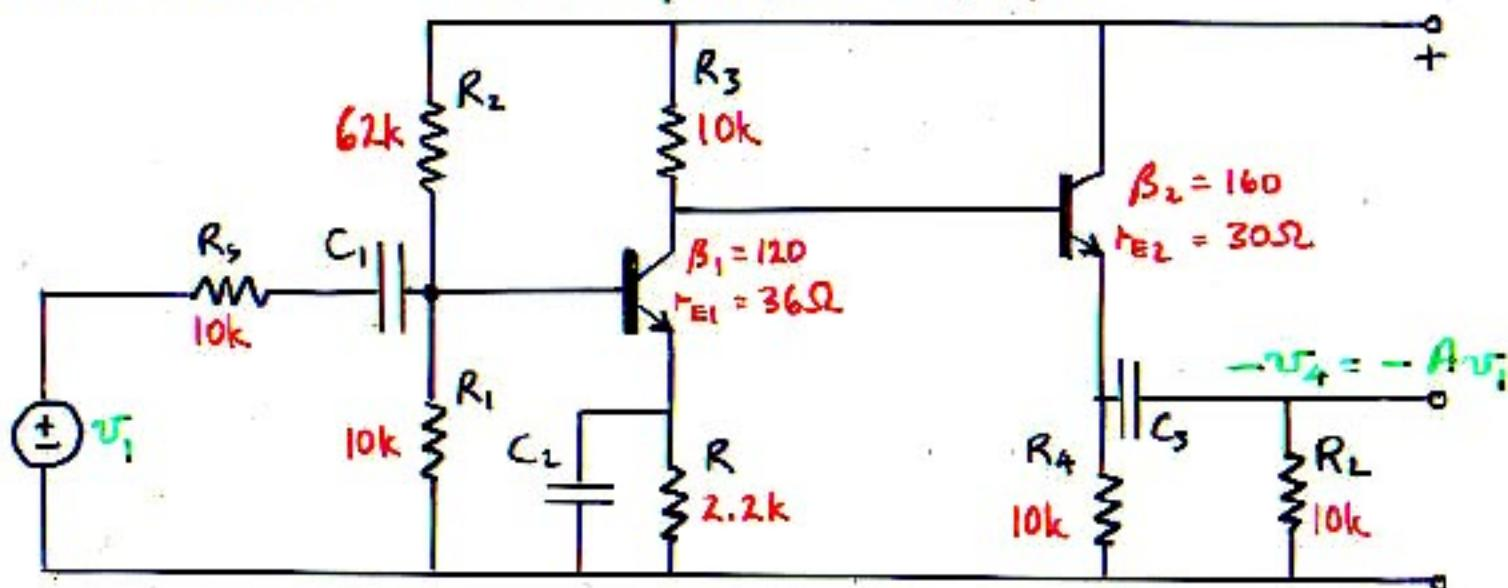
Find the midband gain  $A \equiv v_o/v_i$  analytically and numerically.
