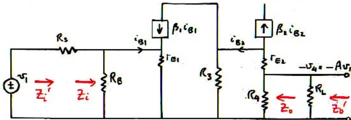
$$A_m = \frac{R_B}{R_B + (1+\beta_1)r_{E1}} \cdot \frac{\beta_1 R_B}{R_s + R_B \parallel (1+\beta_1)r_{E1}} \cdot \frac{R_4 \parallel R_L + r_{E2} + R_3 / (\mu\beta_2)}{R_4 \parallel R_L}$$
