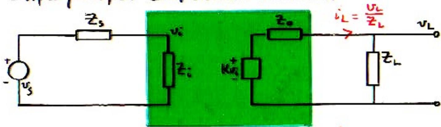
$$\frac{Kv_i}{Kv_i/z_0} = z_0 = \frac{v_L|_{z_L \rightarrow \infty}}{i_L|_{z_L \rightarrow 0}}$$
