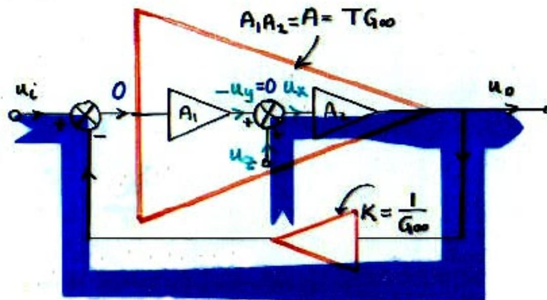
For double injection,  $u_i$  and  $u_z$ , adjusted to null  $u_y$ :
