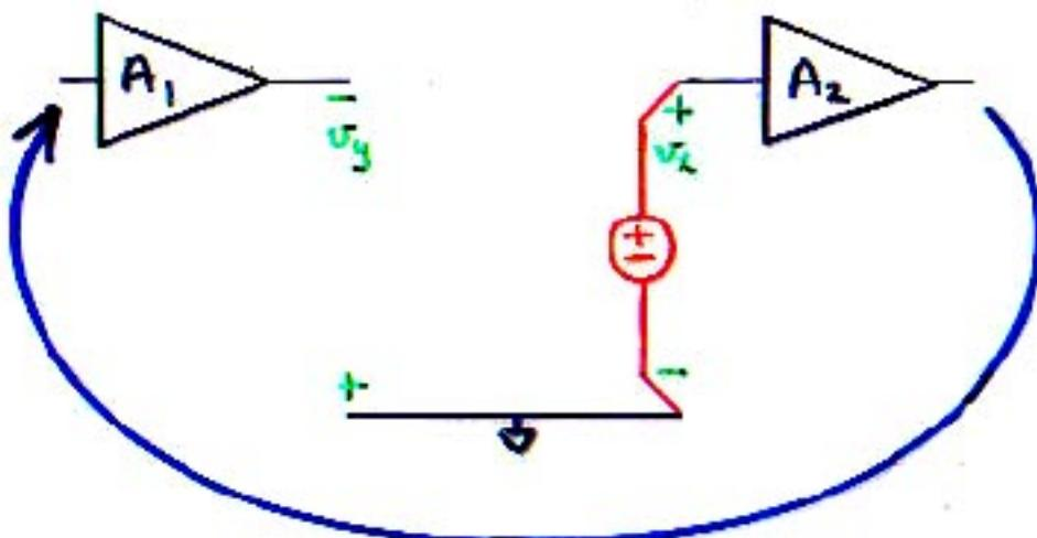
If  $A_1$  and  $A_2$  are unaffected by breaking the loop between  $A_1$  and  $A_2$ , a test signal  $v_x$  may be applied at the input of  $A_2$ , and the resulting signal  $v_y$  at the output of  $A_1$  gives the correct value of the loop gain  $T$  as
