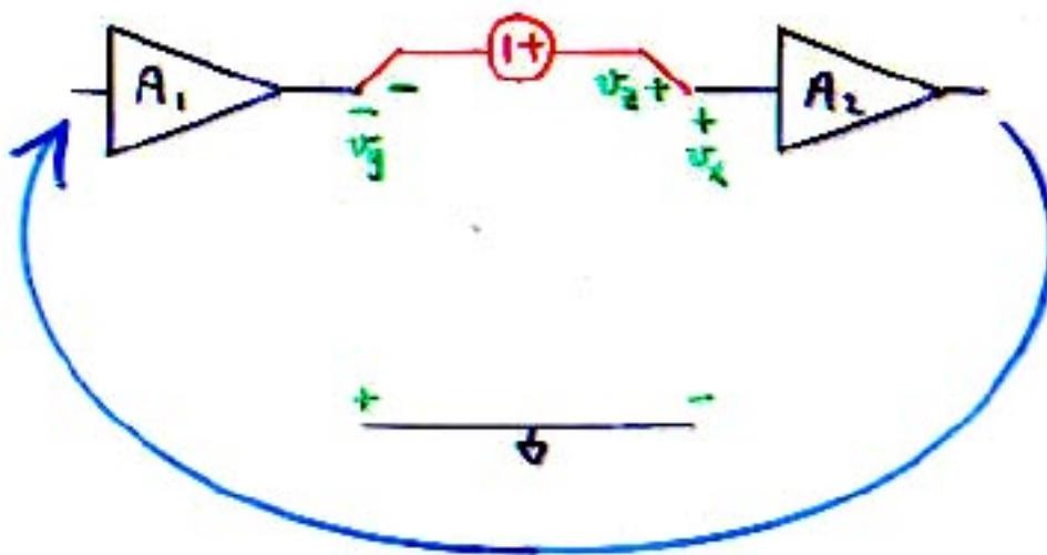
Under such conditions, a voltage  $v_z = v_x + v_y$  exists across the break.
