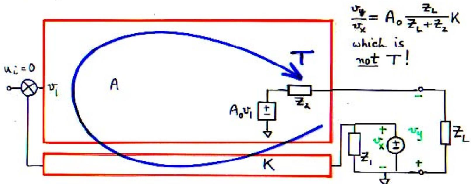
Conventional procedure: break the loop at the output (or input) of the forward path, and find  $T = \frac{u_y}{u_x} = AK$ .
