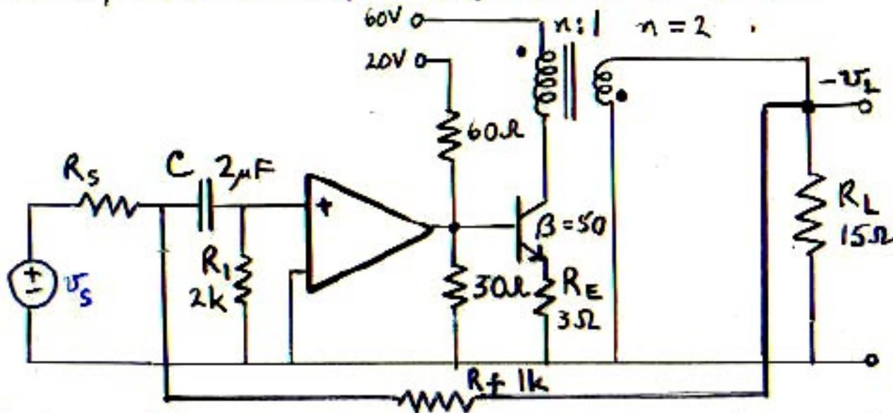
Although the gain is expressed as a voltage ratio, this is really a "Type 3" current-to-voltage feedback amplifier, because the feedback signal is connected at a shunt current-summing junction.
