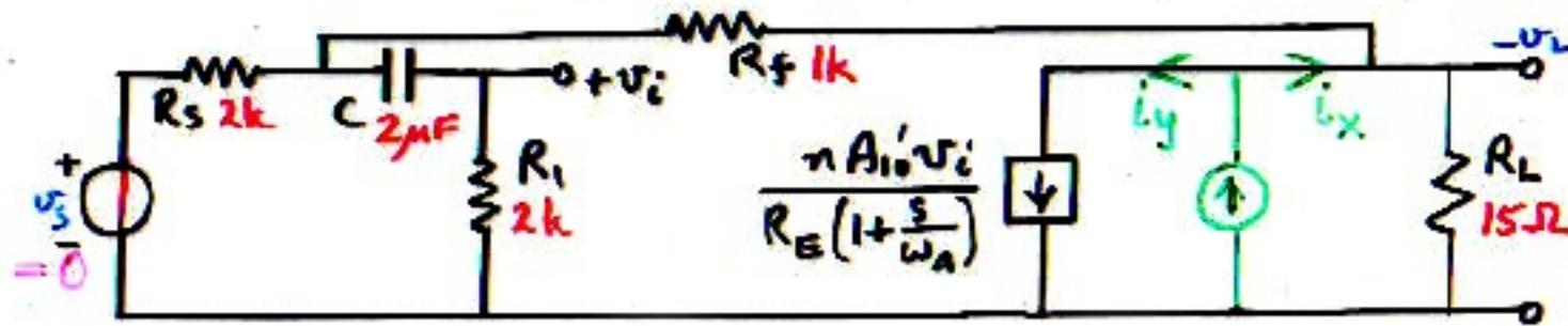
$$T = \left. \frac{i_y}{i_x} \right|_{u_s=0} = \frac{R_L}{R_L + R_f + R_s || R_1 (1 + \frac{\omega_1}{s})} \frac{R_s}{R_s + R_1 (1 + \frac{\omega_1}{s})} \frac{R_1 n A_{10}}{R_g (1 + \frac{s}{\omega_A})}$$
