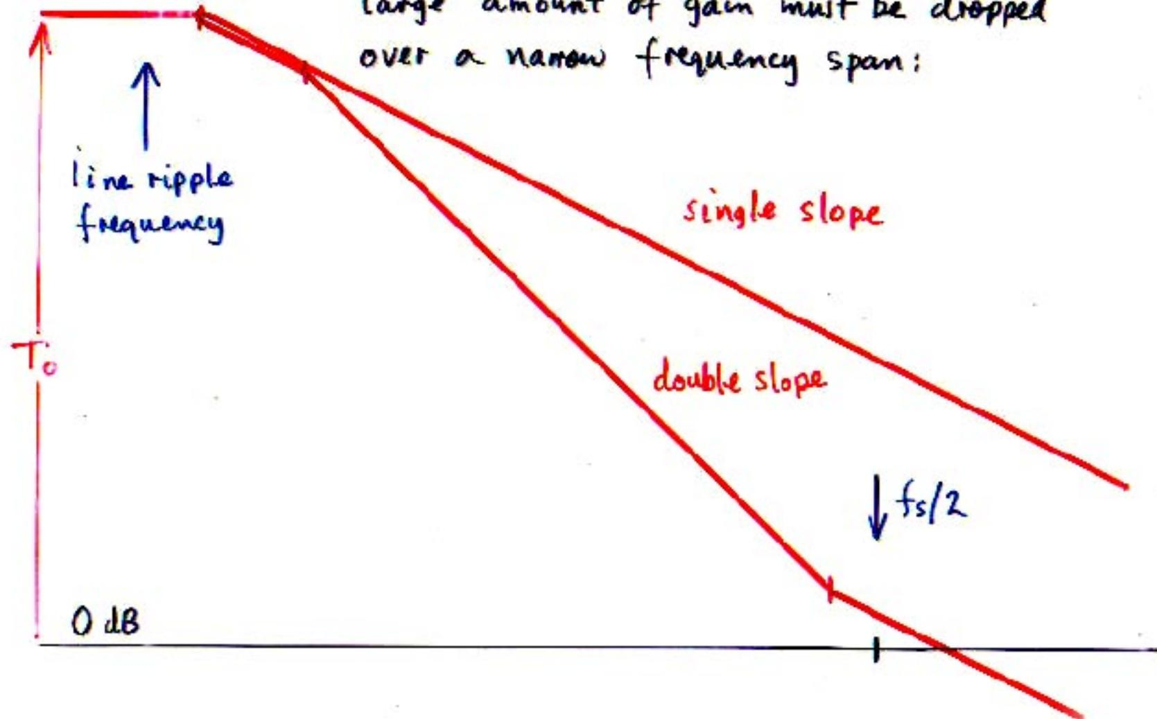
A conditionally stable system may be necessary when a large amount of gain must be dropped over a narrow frequency span:
