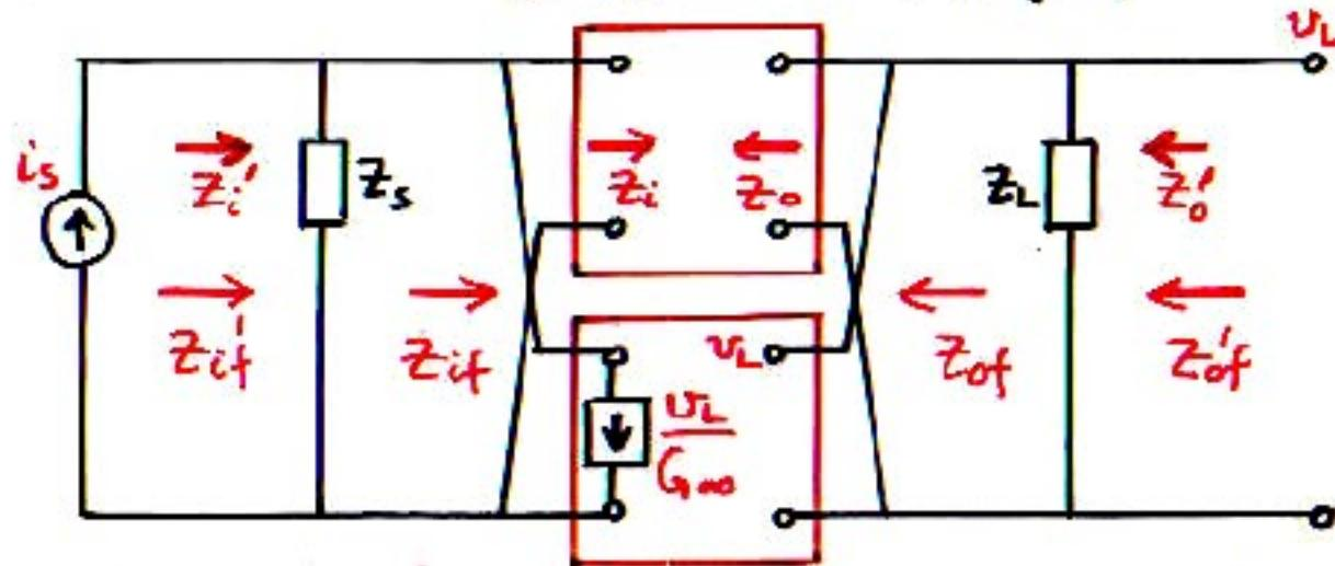
Ideal feedback path must "sense" output voltage and convert it to a feedback current. Current summing is done in shunt.
