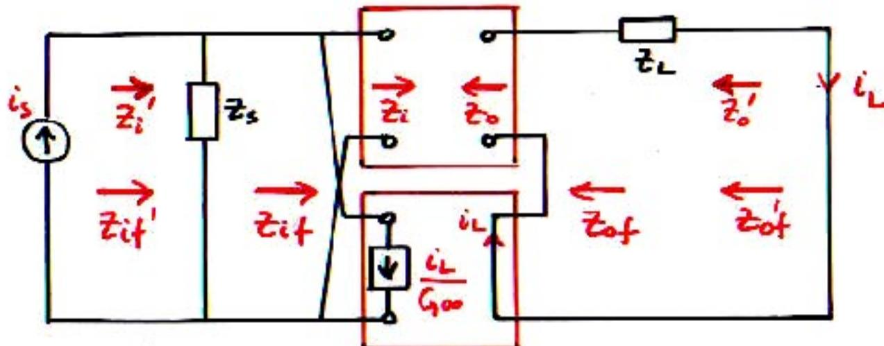
Ideal feedback path must "sense" output current and convert it to a feedback current. Current summing is done in shunt.
