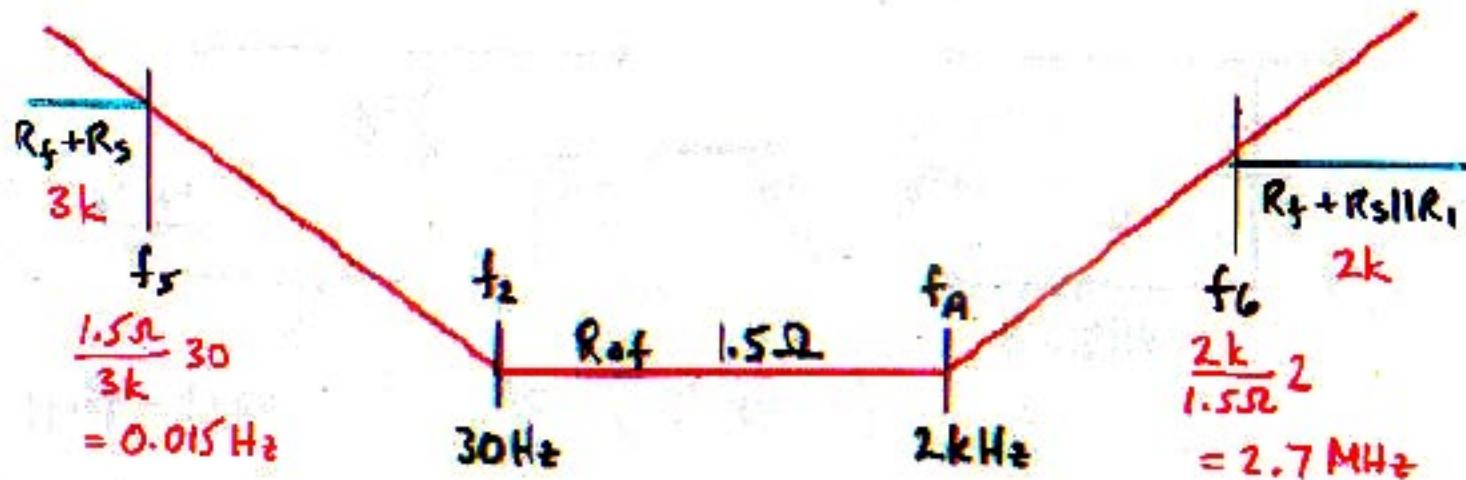
Note from the actual circuit that  $Z_{af}$  would limit at both low and high frequencies, because of the loading effect of the feedback path on  $R_L$ . This nonideality was ignored in the solution, but could have been included with further complication but no additional difficulty.
