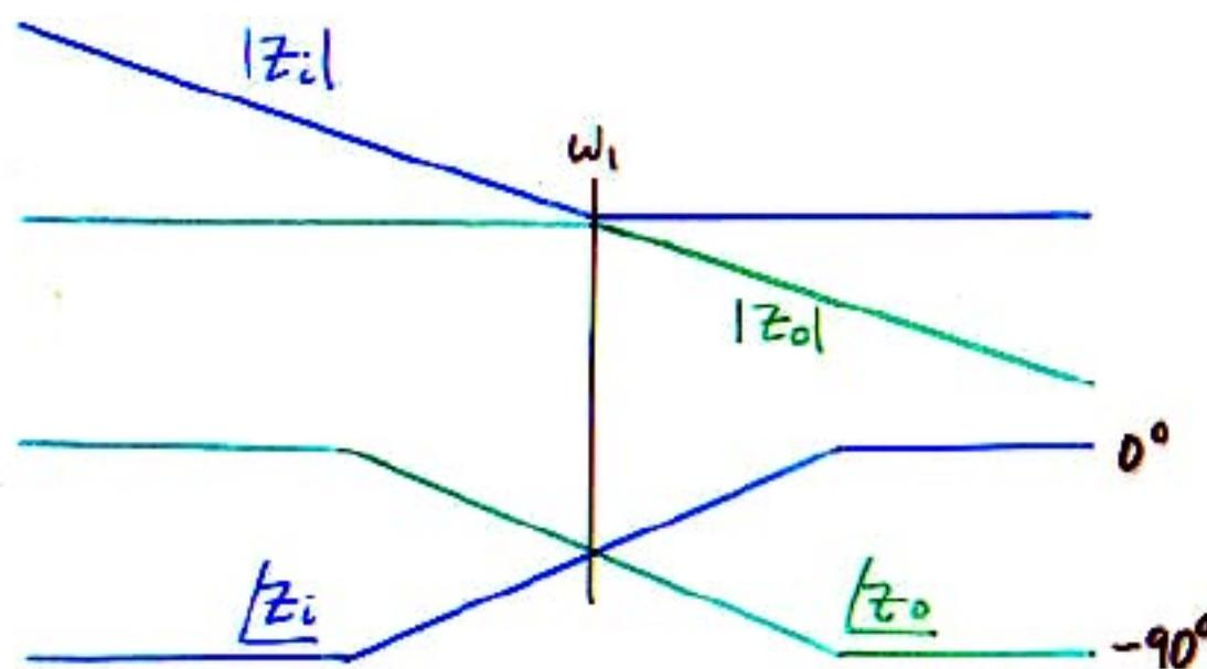
$$\begin{aligned} Z_i &= R + \frac{1}{sC} \\ &= R \left( 1 + \frac{\omega_1}{s} \right) \quad \omega_1 = \frac{1}{CR} \end{aligned}$$
