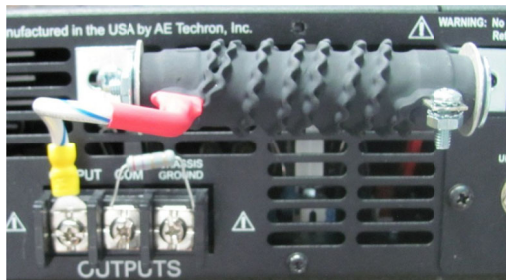
Figure B.2.18 – Connecting the Ballast Resistor Disable Gain Controls
