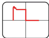
Figure 7.19 – Square Wave Showing a Decrease in R is Required
