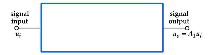
The input is an independent signal, the output is a proportional dependent signal.
