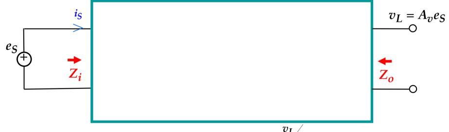
$$Z_i = \frac{\text{input voltage}}{\text{input current}} \quad \text{for the same } v_L$$
