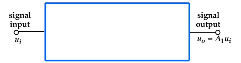
The input is an independent signal, the output is a dependent signal. The gain is  $A_1$ .
