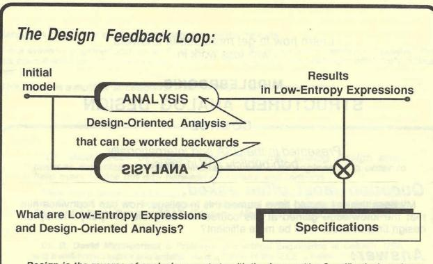
Design is the reverse of analysis: one starts with the Answer (the Specification), and one has to work back to the beginning (circuit configuration and element values). Therefore, only analysis that <u>can</u> be worked backwards is worth doing. This is Design-Oriented Analysis.
