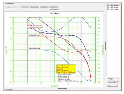
Graph documentation features include Graph Title, Graph Legend, Slide Bar Cursor, and the Data Set Description. The slide bar cursor is an especially useful tool for displaying specific data on a graph.
