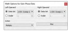
Venable's Stability Analysis Software allows the user to manipulate, display and import/export data. The "File Math" function allows any kind of mathematical function on any one or two transfer functions (measured data sets).
