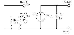
This is a current source controlled by the voltage from node 3 to node 4. It has a gain of 0.1, which means 1 volt from node 3 to node 4 will produce 0.1 amp from this source. It is connected in the circuit from node 2 to node 0, and is paralleled by a 1 mega-ohm resistor. Node 2 is in phase with node 3.
