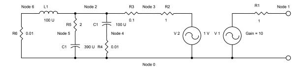
Normally R3 would be 1 ohm to simplify the calculation, and V1 would have a gain of 1. The values used in this example show the flexibility of the technique.
