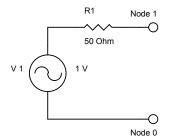
This is a fixed 1-volt source with an impedance of 50 ohms, connected in the circuit from node 1 (positive node) to node 0 (negative node). Node 0 is always circuit common.
