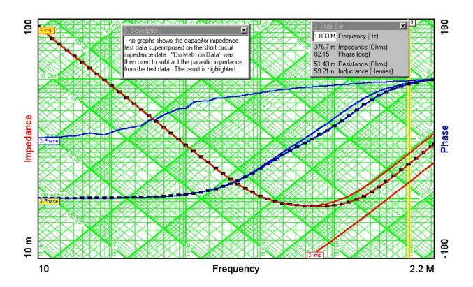
The example on the previous pages was for measuring a low impedance and correcting for short circuit parasitics by subtracting the short circuit impedance from the test data. The same concept can be used for measuring high impedances and correcting for open circuit parasitics, except it is a little trickier because the open circuit parasitics are in parallel with the test data instead of in series.
