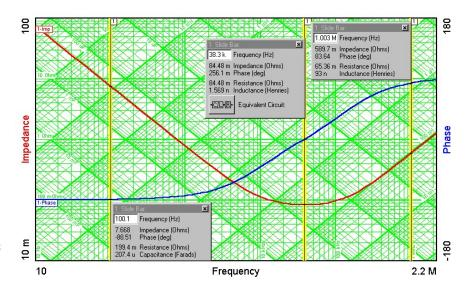
voltage of 35 VDC and a nominal capacitance value of 200  $\mu$ F. We added slide bars to show the capacitance at 100 Hz (207.4  $\mu$ F), the ESR when it is purely resistive (84.48 milliohms), and the inductance at 1 MHz (93 nH).
