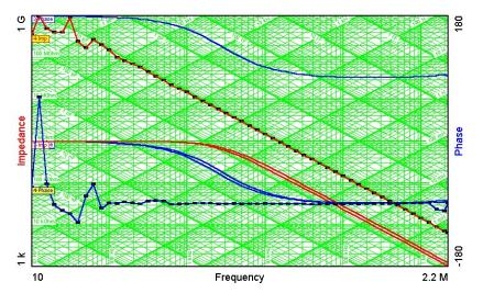
mega ohms. Beyond that, the data is noisy because the parasitic resistance is only 1 mega ohm. At the upper left corner of the graph we are trying to resolve the difference between 1 mega ohm and 1 giga ohm in parallel with 1 mega ohm, and understandably the result has a little variance because we are approaching the limits of measurement resolution.
