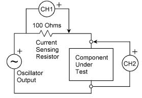
(CH1) "backward", so the return is connected to the oscillator output as shown in the figure. This minimizes the parasitic capacitance across the component under test.
