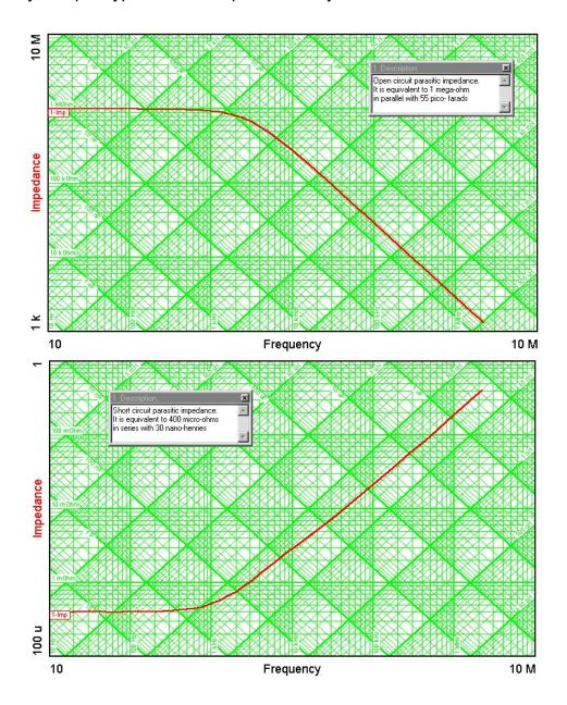
The graph below shows the result of using "Math Options for Impedance Data" to subtract the parasitic short circuit impedance from the capacitor impedance test data. The impedance is too far below the open circuit impedance to require compensation for open circuit parasitics. The true inductance of the capacitor can be seen in the text box near the slide bar to be 59.21 nH instead of the 93 nH we measured without correcting for short circuit parasitic impedance.
